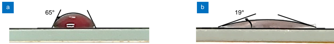
Fig. S1 | Images of water contact angles on (a) pristine and (b) laser sintered GWLM films.
