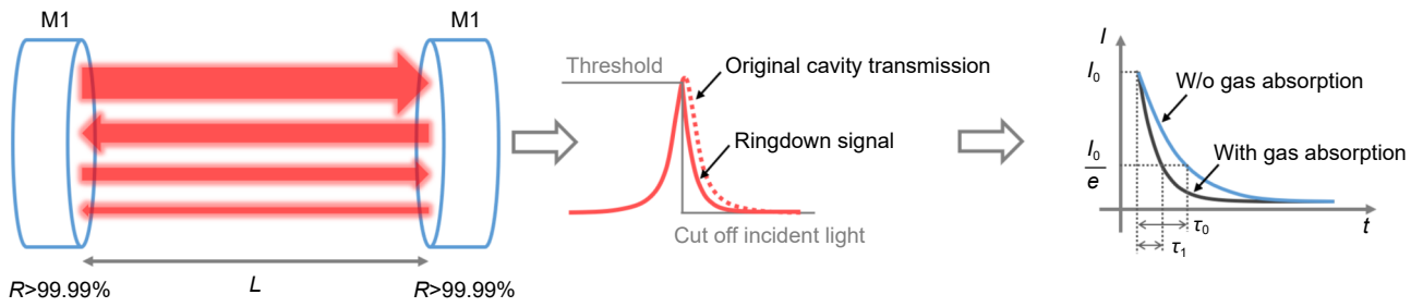
Fig. S2 | Schematic of cavity ringdown spectroscopy. R , reflectivity of the cavity mirror; L , physical distance between two cavity mirrors; I , intensity of the cavity-transmitted light detected by photodetector; I_0 , cavity-transmitted light intensity at the moment when the incident light is cut off; \tau_0 , ringdown time of the cavity without gas absorption; \tau_1 , ringdown time of the cavity with gas absorption.
