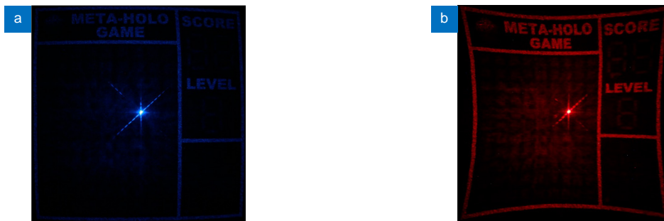
Fig. S2 | The experimental result plots with more obvious pattern distortion at (a) 473 nm and (b) 633 nm, respectively.
